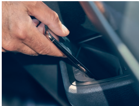
Station de recharge inductive 6)
